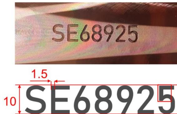
**Figure 1. Example of engraved identifier on a copper sample. The measures of the characters are shown below.**
