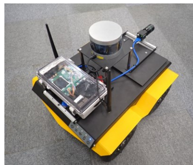
Fig.2. An unmanned ground vehicle (Jackal, Clearpath robotics) equipped with a CsI scintillation detector, a GPS, a LiDAR, and a camera.
