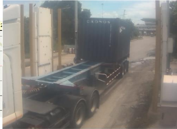
Figure 6. Improper background updating caused by a truck stopping at the RPM. In this case, the open flatbed section contributed to the first occupancy ending, allowing a second occupancy to begin without the truck exiting the RPM.
