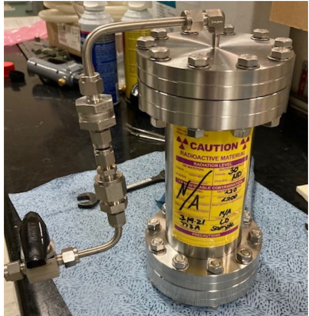
Figure 1. Sealed mini-canister for aluminum radiolysis campaign (with markings for a contaminated sample) showing sampling tube attached to lid.
