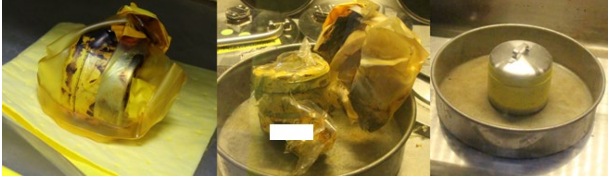
Figure 4 - (left) 1/4 Qt inner slip lid, (middle) bag condition and content verification, (right) new taped slip lid after repackaging.
