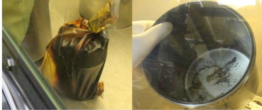
Figure 2 - (left) "Hatch" material contained in a conflat package bagged out in a sPVC bag. (right) Residue and corrosion on the interior walls of the outer 5 Qt Hagan container.
