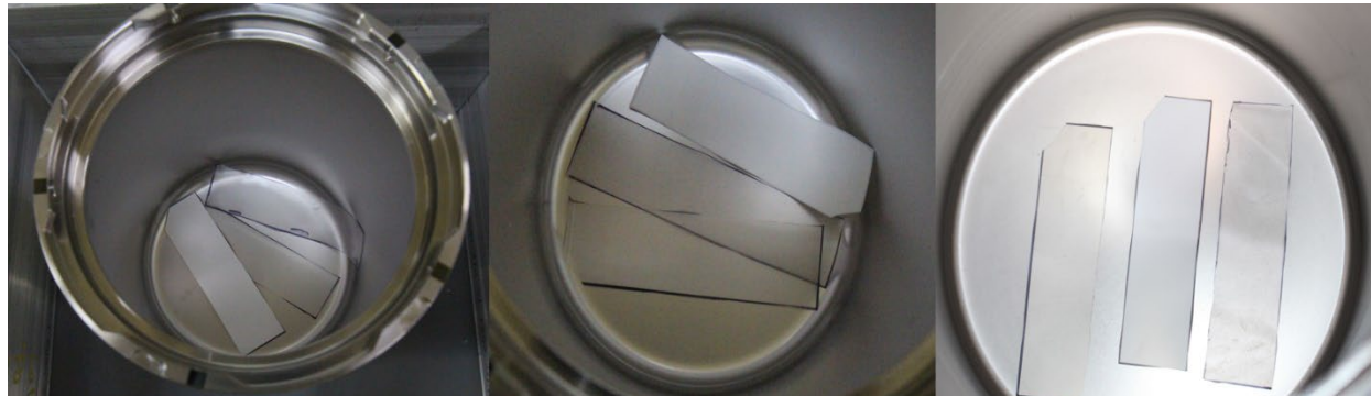
Figure 1- Placement of material samples in the SAVY container of various sizes
