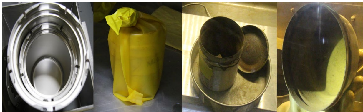
Figure 6 - From left to right: Interior pictures of the outer 3 Qt SAVY-4000, APU-E bag-out bag, slip lid inner container, lid of the inner container exhibiting general corrosion.
