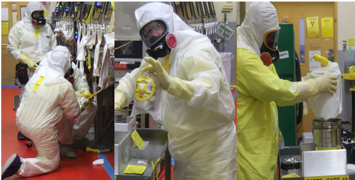
Figure 8 - Glovebox fissile material handlers conducting bag-outs of the APU-e items.
