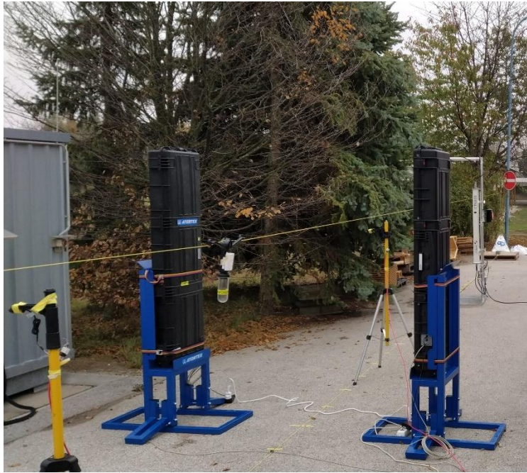
Figure 1. Remote control camera slider being used as a linear motion device for dynamic response tests of relocatable RPMs.
