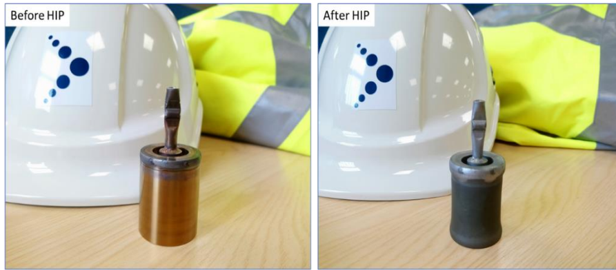
Figure 4: Small scale (44 g loaded) HIP canister before and after HIP.
