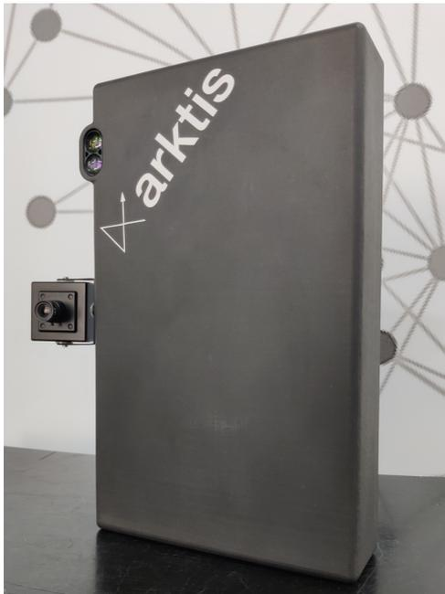
Figure 1. The Flat Panel Gamma detector by Arktis Radiation Detectors comprises flat scintillator panels read out by solid state “Silicon Photomultiplier” electronics.
