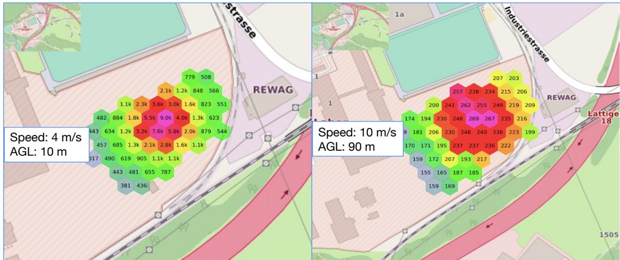
Figure 6. Scenario B. Cs-137 source search missions performed with a low-speed, fine scan (left) and with a high-speed, coarse scan (right).
