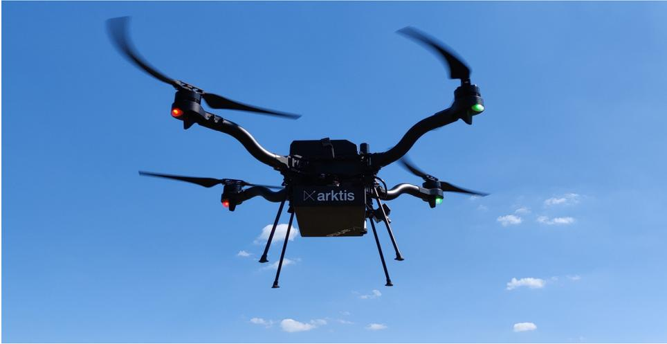
Figure 2. Astro drone equipped with the FPG detection system offers high sensitivity for a system its size.
