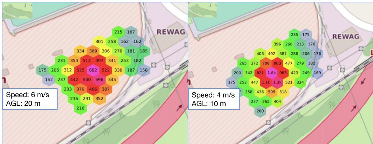
Figure 10. Count rate heatmap generate in scenario D flight missions. Hotspot shows the position of the Ba-133 radionuclide source.
