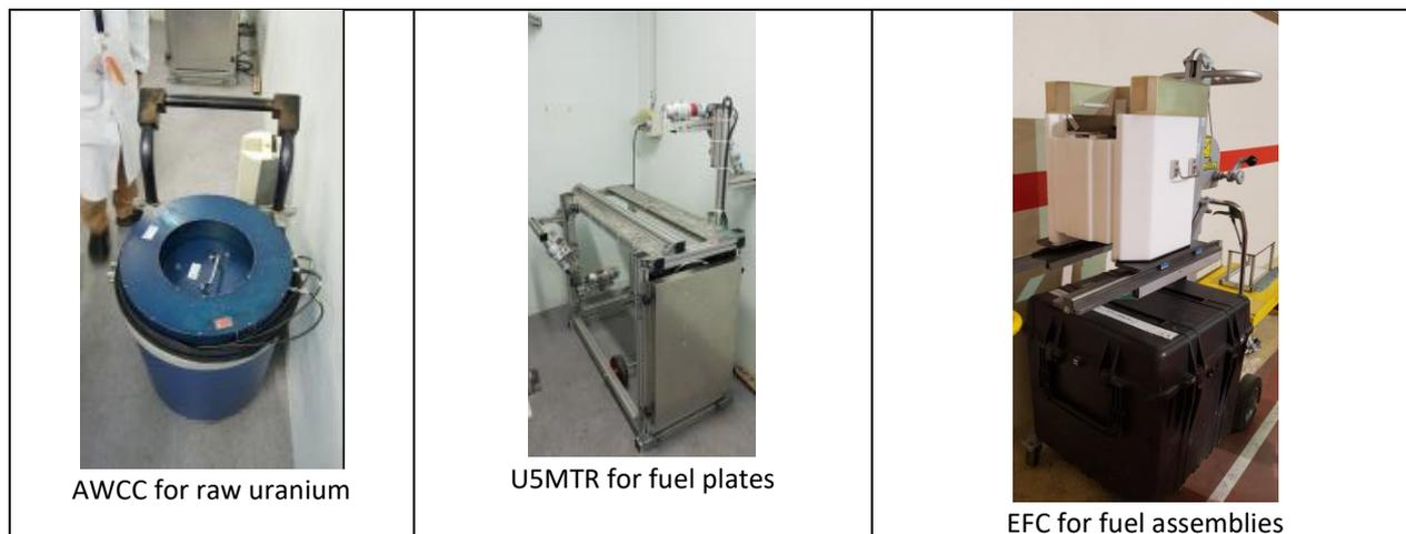
Figure 9 – Main verification devices used by Euratom in Framatome facilities. © Framatome
