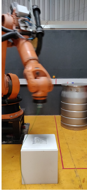
Figure 6: Image captured during a run of the KUKA robotic arm manipulator with a CsI(Tl) detector attached, moving over a 370 kBq Cs-137 source in a 0.5 cm thick lead casing.
