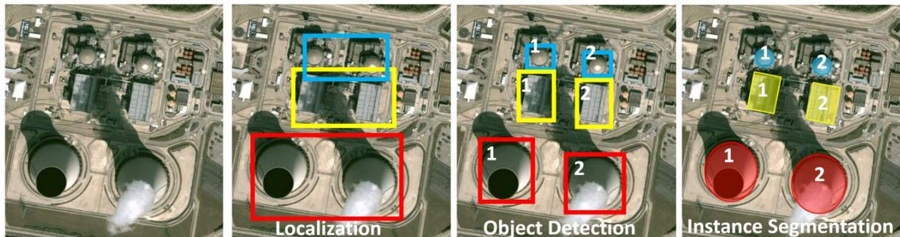
Figure 3. Illustration of localization, object detection and instance segmentation of different components of the nuclear power plant shown in Fig. 2. Red highlights cooling towers, yellow outlines turbines, and blue outlines reactors. Numbers represent IDs of individual instances of cooling towers, turbines, and reactor buildings. Image credit © Google Earth.
