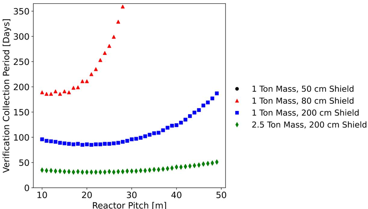
Figure 4: The collection period required for power verification with varying reactor pitches and detector configurations. The antineutrino detector is assumed to be placed directly in the middle of the reactor hall and the misused reactor core is assumed to be an innermost core
