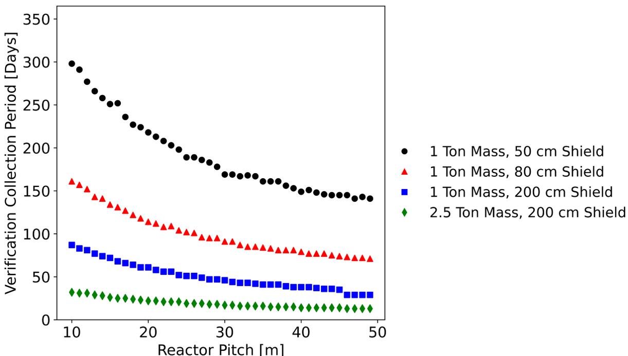
Figure 5: The collection period required for power verification with varying reactor pitches and detector configurations. The antineutrino detector is assumed to be placed directly across from the misused reactor and the misused reactor core is assumed to be an innermost core
