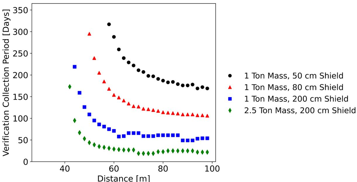
Figure 2: The collection period required for power verification with varying background collection standoff distances and detector configurations
