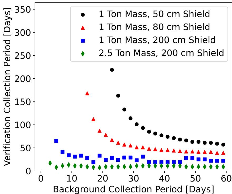
Figure 1: The collection period required for power verification with varying background collection periods and detector configurations
