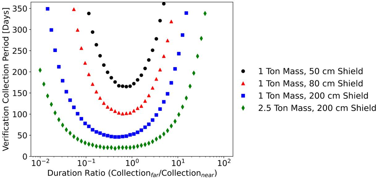
Figure 3: The collection period required for power verification with varying duration ratios and detector configurations
