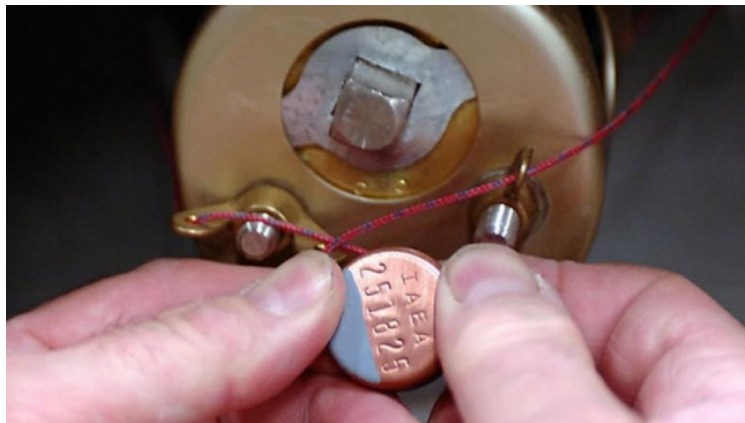
Figure 1: Cap Seals used by IAEA ( https://www.iaea.org/newscenter/news/safeguarding-the-future-iaea-looks-for-improved-solutions-for-passive-loop-seals-for-nuclear-verification )
