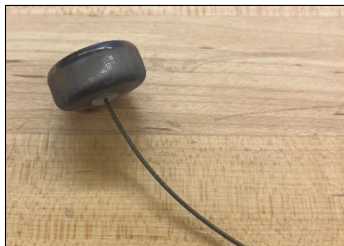
Figure 8: 3D-printed body with plug inserted and wire penetrating through the plug. Picture from SNL.
