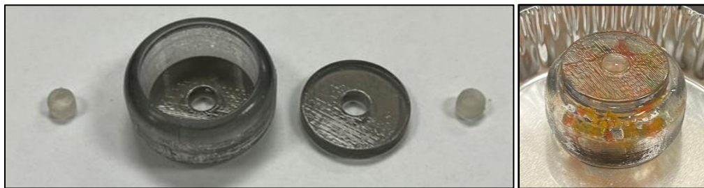
Figure 7: (Left) 3D-printed outer shell with single hole for plug testing, (Right) assembled seal body with inner sensing mixture included. Pictures from SNL.
