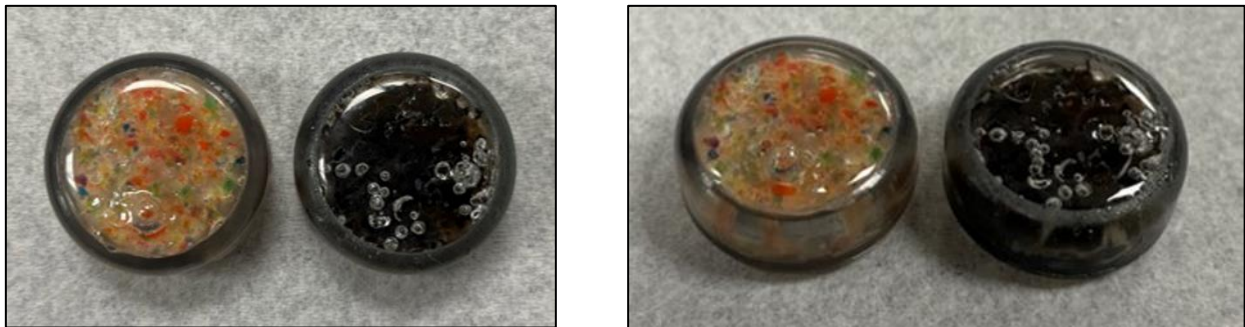
Figure 4: (left of each image) Material samples showing outer shell and inner sensing mixture; (right of each image) material samples demonstrating tamper event, which causes seal to irreversibly turn black. Note the unique identifier patterns formed from both the colored water beads and the bubbles. Pictures from SNL.
