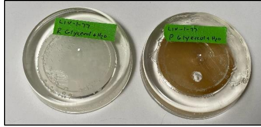
Figure 5: Material samples from prior Bleeding Materials project, whose goal was to develop tamper-indicating enclosures with visually obvious tamper response. (Left) untampered sample, (right) sample after drilling into inner sensing mixture (tampering). Pictures from SNL.
