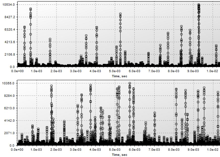
Figure 2. Waveforms acquired from a subcritical ( $k_{eff} = 0.9948$ , top) and critical (10 mW, bottom) reactor.
