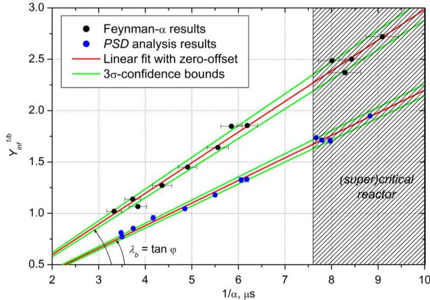
Figure 3. Results of the neutron noise measurements at the TAPIRO reactor. The error bars represent statistical uncertainties with coverage factor  $k=3$ . The shaded area highlights the domain of the reactor (super)criticality.
