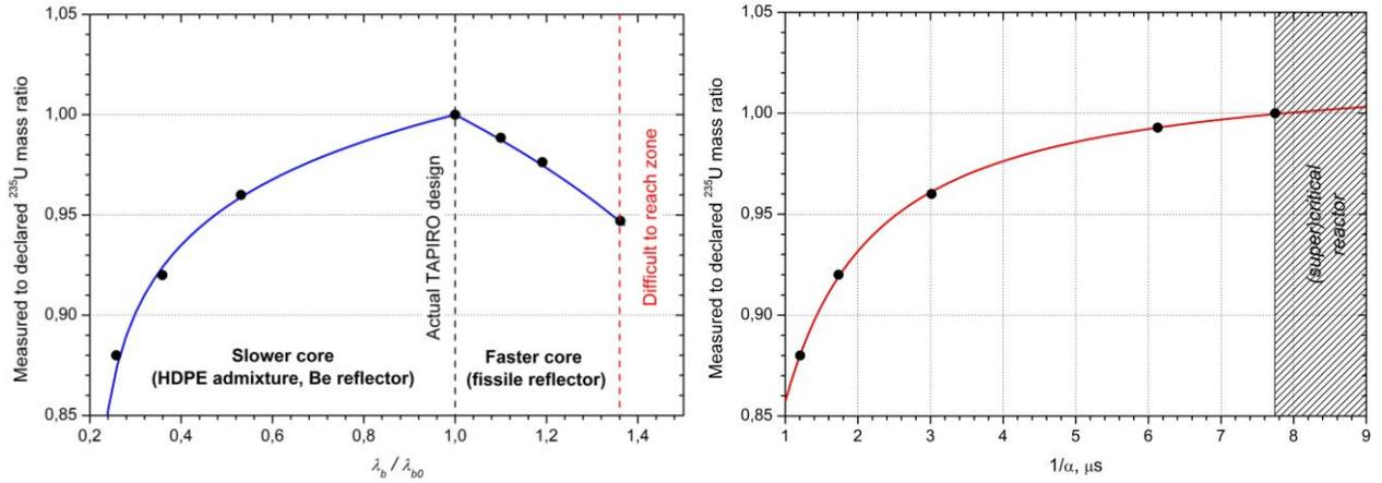
Figure 5. The  $\lambda$ -calibration (left) and  $\alpha$ -calibration (right) curves for the TAPIRO reactor.
