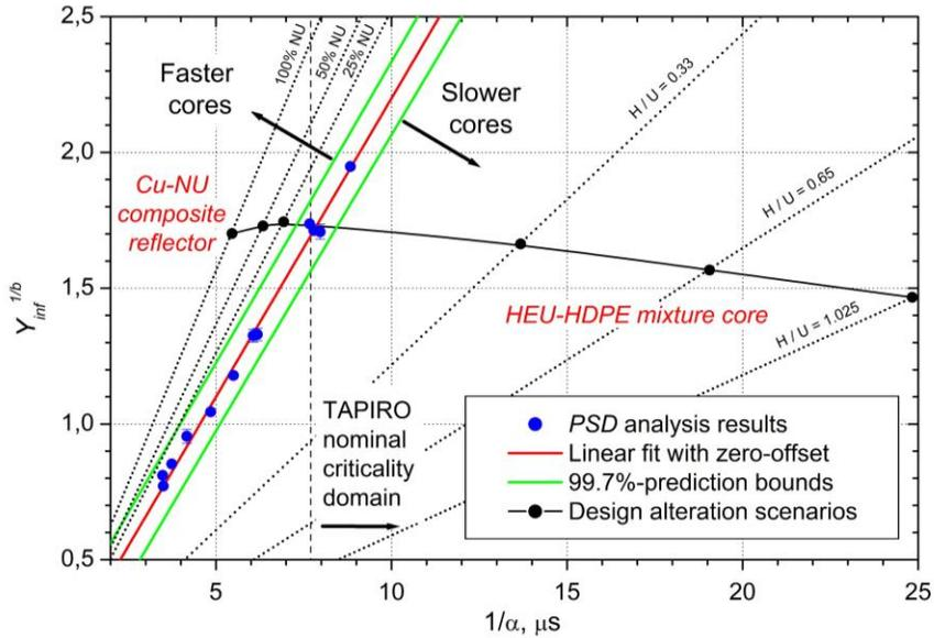
Figure 4. The  $Y_{\infty}^{1/b}$  vs.  $\alpha^{-1}$  plot combining the results of the PSD analysis of the neutron noise measurements with the results of the sensitivity study for two design alteration scenarios: (i) neutron moderation in a mixed HEU-HDPE core, and (ii) neutron multiplication in a composite Cu-NU reflector.
