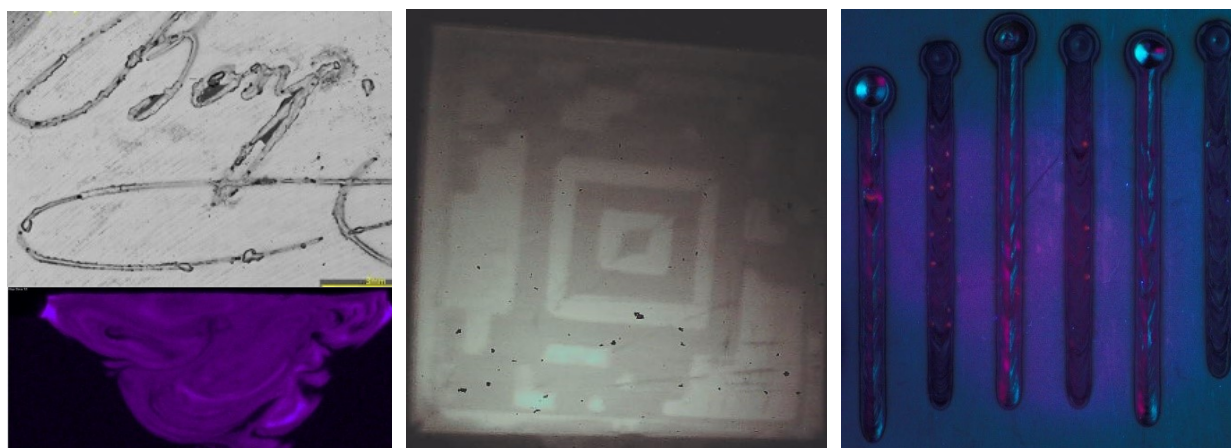
Figure 6. Examples of surface tagging. (left) A signature applied by laser deposition of titanium foil onto 304L stainless steel, with its cross-section mapped by SEM-EDS in the lower panel. (center) A 2-dimensional code applied by atomic layer deposition of zirconium oxide ( ZrO_2 ) on an aluminum surface, visualized under UV irradiation. (right) Photoluminescence of europium oxide ( Eu_2O_3 , left) and aluminum oxide ( Al_2O_3 ) particles embedded in 304L stainless steel by weld deposition.
