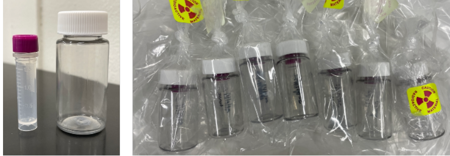
Figure 2: Samples prepared for gamma measurements consisted of 1.5 mL total solution volume in a plastic vial, overpacked in a plastic scintillation vial and plastic bag. Image on left shows empty vials for reference.
