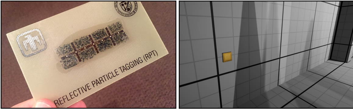
Figure 5: A “virtual peephole” into the physical world from within virtual reality could allow inspectors to verify the integrity of a unique identifier previously installed in the facility (left). Such a “virtual peephole” could be shown in virtual reality in some form, such as a limited video transmission. The golden plaquette (right) is a placeholder for such a peephole. Source: Authors.
