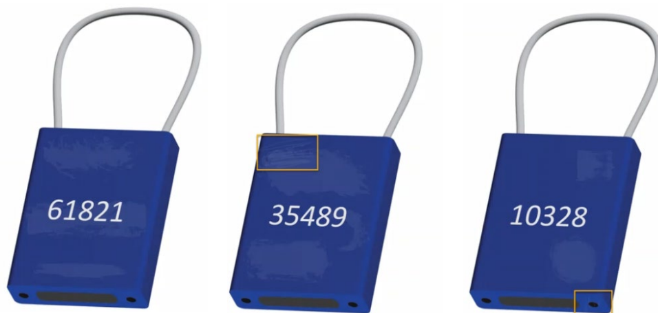
Figure 1. Example Tamper Manipulations. From left to right: Normal wear and tear (no tamper), tamper in top left corner (highlighted in yellow), tamper on bottom of the seal, right corner (highlighted in yellow).
