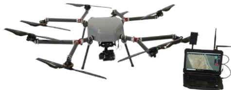
Figure 3. Skyfront Perimeter 8 Hybrid Fuel UAS (unloaded flight time of five hours)
