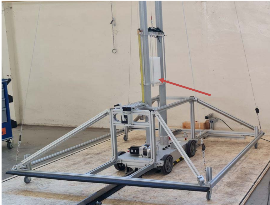
Figure 1: Dynamic test system with neutron source behind HPDE shielding, see arrow.
