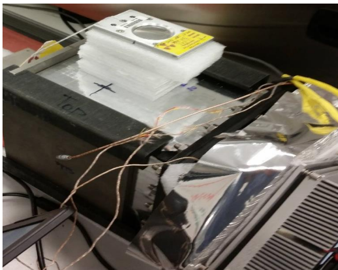
Figure 7. Detector tested on a ^{238}\text{U} source.
