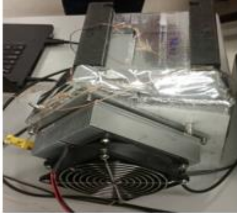
Figure 3. Cooling system attached to detector and outside box.
