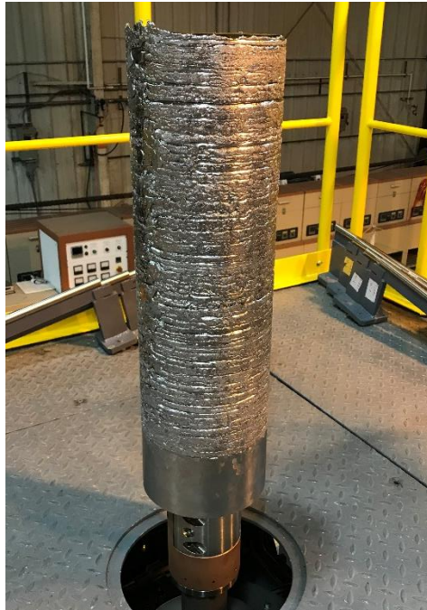
Figure 6. Ti-Nb Ingot Produced in NIMF Furnace Placed Based on Agile Effort
