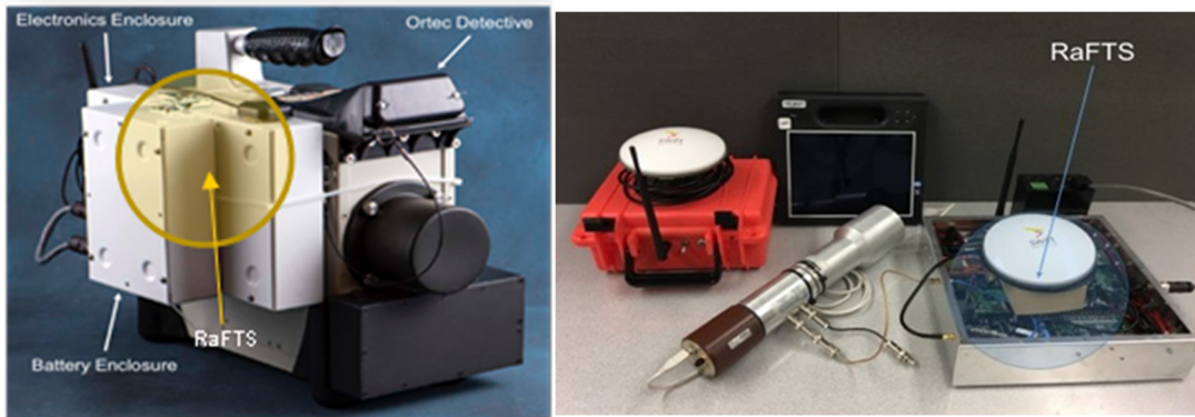
Figure 1: RaFTS operates on different spectrometer systems: (Left) on a commercial semiconductor-based system, the Ortec Detective; and (Right) a commercial sodium-iodide-based detector. The flexibility of RaFTS for different types of detector instruments makes this innovation an attractive commercial product for the rad-nuc safety sector.
