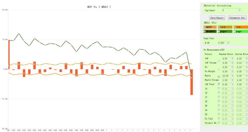
Figure 5b The Traditional Accounting Result of Plutonium in MBA2
