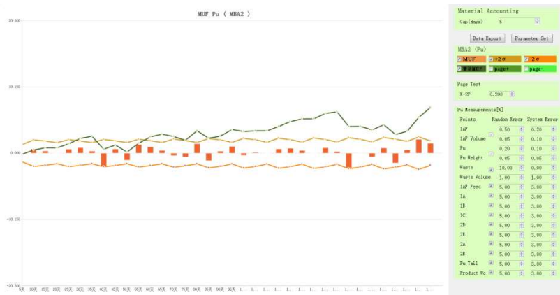
Figure 5a The Near Real Time Accounting Result of Plutonium in MBA2
