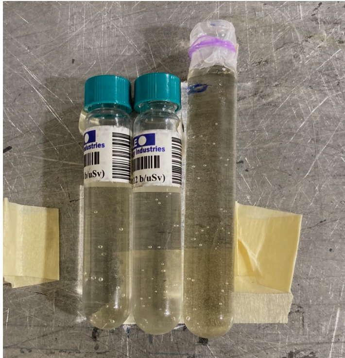
Figure 2. Droplet detectors showing bubbles formed after being exposed to ^{252}\text{Cf} .
