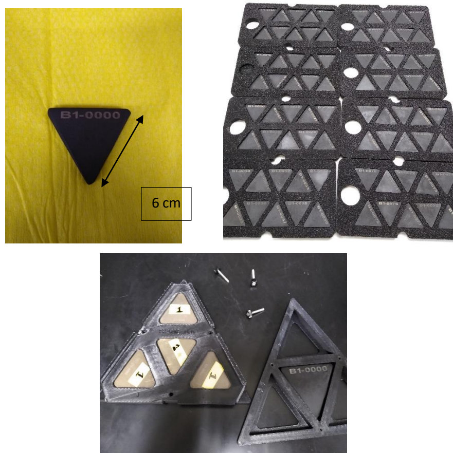
Figure 2. New components. Top left , A single DU triangle with unique identification. Top right , The complete inventory of 80 DU triangles in their holders. Bottom , The new quad triangle assemblies hold two layers of tiles. The example shown includes one inner layer of DU tiles and one outer layer of HEU tiles
