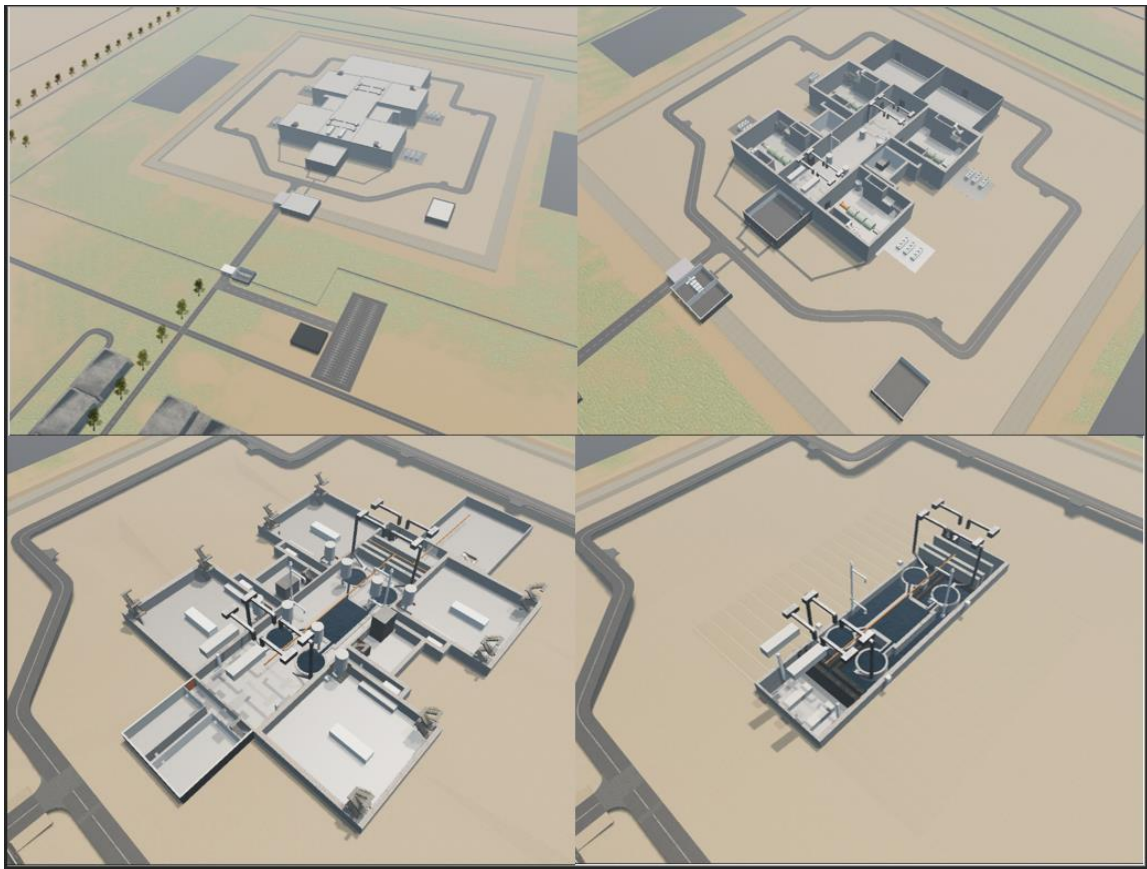
Figure 1 Hypothetical SMR Facility. Above-grade (top left), basement one (top right), basement two (bottom left), basement three (bottom right).
