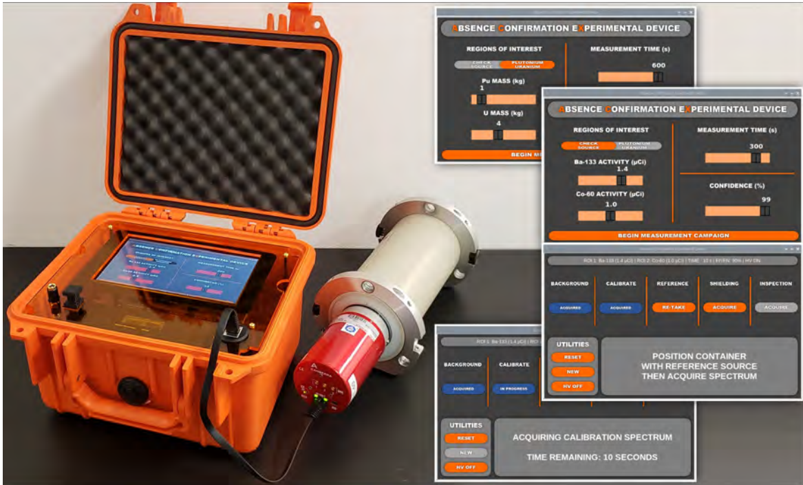
Figure 3: Absence confirmation device with sample screenshots. The ACX (Absence Confirmation eXperimental) device is shown connected to a collimated NaI detector. A custom GUI guides the inspector through the verification protocol. The start screen is shown in the upper-right, which can be toggled to operate with special nuclear material or laboratory check sources. In the lower-right are two sample screenshots of the GUI at various steps during the protocol.
