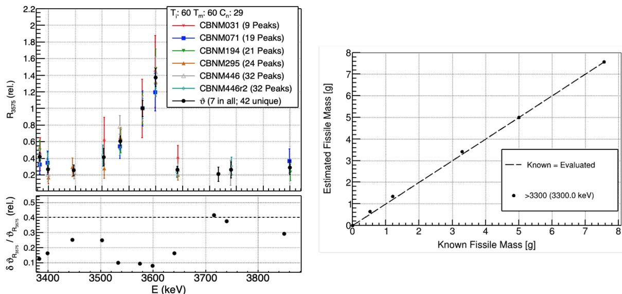
**Figure 2. Fission product gamma-ray peak ratio for composition analysis (left) and integrated counts for mass correlation analysis (right).**
