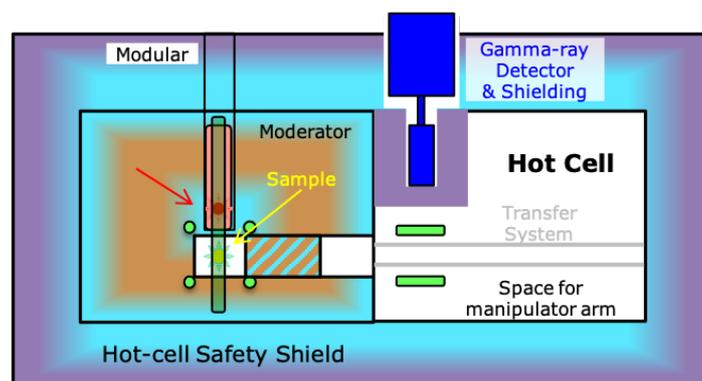
**Figure 3. Preliminary concept for the JAEA/ISCN practical DGS instrument.**
