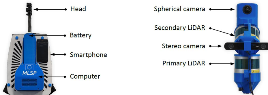
Figure 1. MLSP backpack used for data acquisition. (left) main body of the backpack with the smartphone. (right) Sensors head mounted on the top of the backpack.
