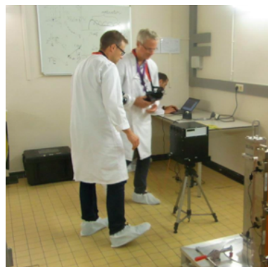
(a) A photo of the nFacet 3D system on a tripod ready to take data with the MOX assembly in front.
