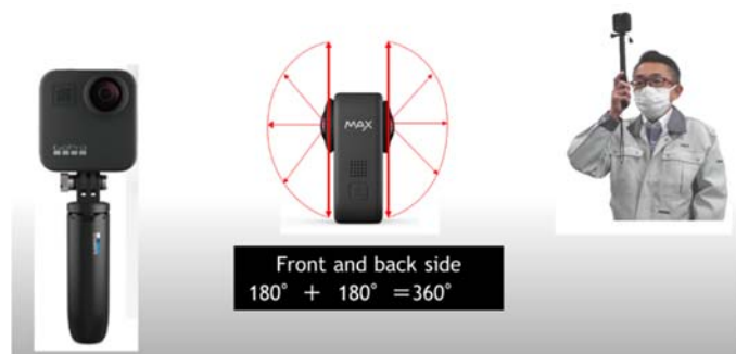
Fig.2 How to take 360-degree pictures
