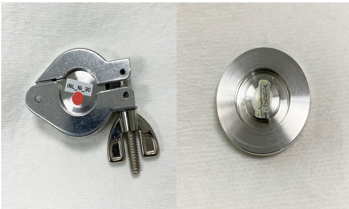
Figure 1. Standard KF-16 flange blanks used as part of the SUDA sampler to collect \text{UF}_6 gas. Right: Nickel foam support containing the collected \text{UF}_6 as uranyl fluoride adsorbed onto zeolite.
