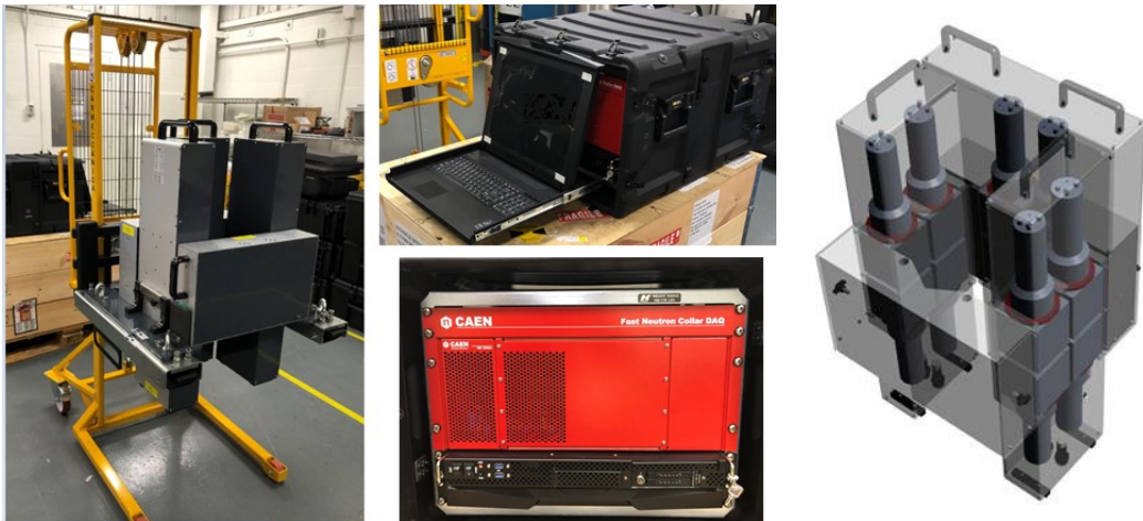
Figure 1. Photograph of the CAEN FNCL detector assembly (left), the acquisition electronics (center), and an isometric view showing the arrangement of the 12 EJ309 neutron detectors [10] (right).
