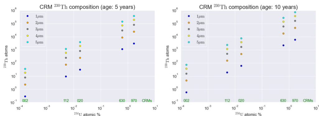
Figure 1. Predicted concentrations of ^{230}\text{Th} for various CRMs with respect to particle size.
