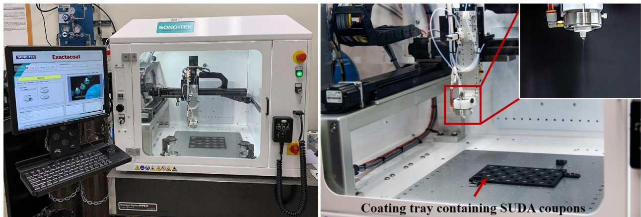
Figure 2. The auto-coating instrument used to coat the absorbent film onto the SUDA substrates (Left). The image on the Right shows the configuration of the instrument for coating and the inset (top right) shows the ultrasonic spray nozzle with fine spray control.
