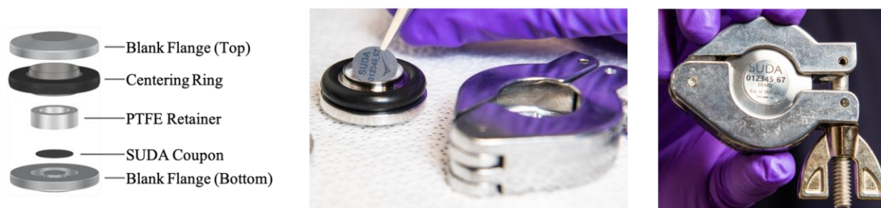
Figure 1. Typical construction of a SUDA sampler, where Left is the expanded view of a SUDA sampler; Center shows a SUDA substrate coated in \text{UF}_6 -absorbent material being loaded into the SUDA sampler (with the labeled back-side facing up); and Right is a fully assembled SUDA sampler.
