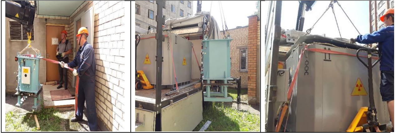
Pic 4. Loading the irradiation head to the KMZ container on the truck.
