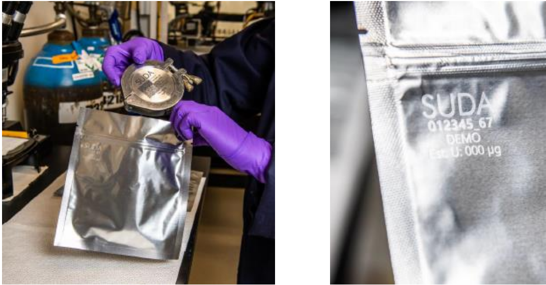
Figure 8 Photograph of a large SUDA sampler being placed in a mylar resealable bag (left) and a close-up image of a laser-etched marking in a mylar bag (right).
