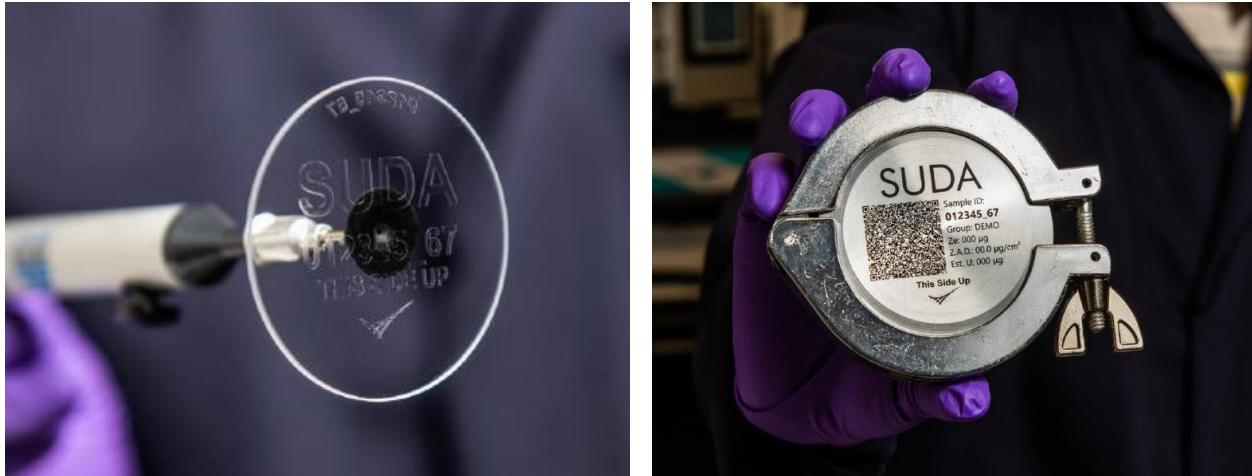
Figure 4 Photograph of the improved SUDA sampler wafer (left), and the new markings on the SUDA sampler's KF flange (right).
