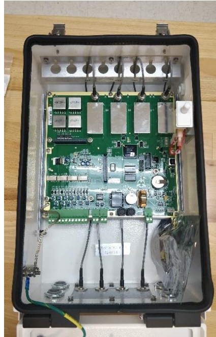
Figure 5. OmniTrax processor with 4 receive and transmit ports inside the enclosure.
